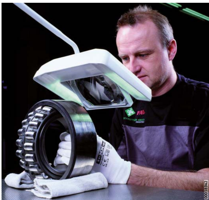
Figure 6 Bearing examination by Schaeffler reconditioning specialists
