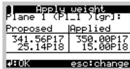
You can abort input of weights at any time by pressing *the Esc button*
