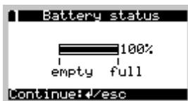
During normal operation, the accumulator symbol (top left of display) indicates the charge level.
