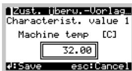
Accept this value by pressing the Enter button
