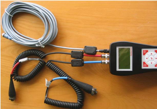
*Ferrites attached to sensor cables*
