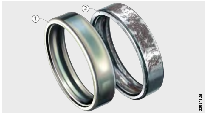
Figure 8 Bearing rings after the salt spray test
