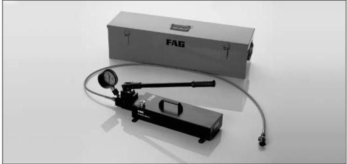
54: FAG Hand pump set PUMP2500.8L.D, consisting of a two-step piston pump (2500 bar) with 8-litre oil container, two-way-valve, manometer, 2 HP tubes, 2 closing nipples G 1/4, 2 adapters and 6 reduction adapters, metal box
