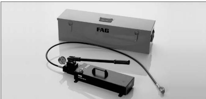
52: FAG Hand pump set PUMP1000.4L, consisting of a two-step piston pump (1000 bar) with 4-litre oil container, manometer, 1 HP tube, plug-in joint (connecting thread G 1/4), metal box
