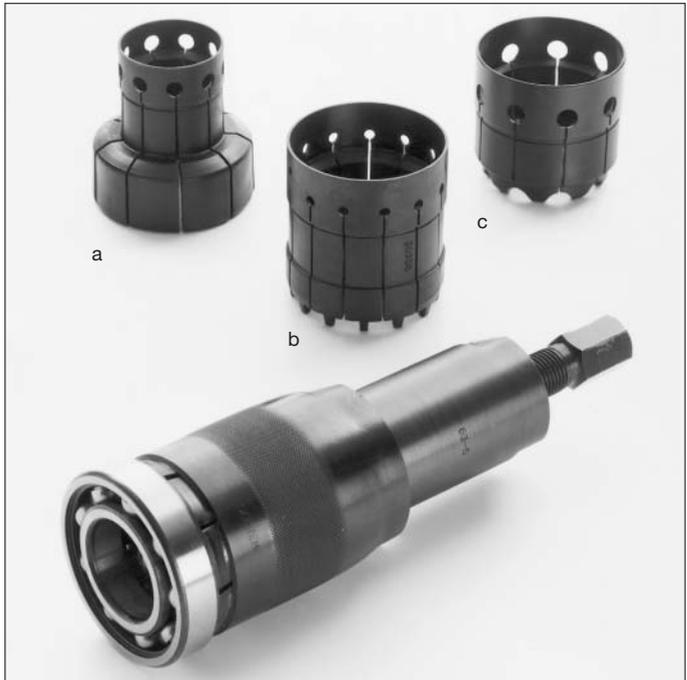
The clamping piece forms part of a collet and is clamped against the inner ring with a tapered clamping ring. The extraction force is generated by a spindle. This extractor enables bearings mounted in the housing to be withdrawn from the shaft.
