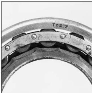
The location of the load zone in a bearing ring results from the direction of the externally applied loads and from the conditions of rotation. The load zone can soon be recognized by slight frosting on the raceways indicating whether the bearing was loaded as specified.
