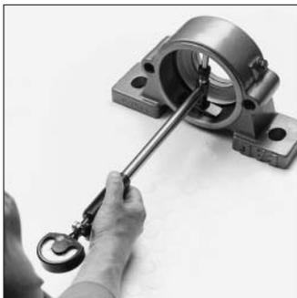
7: Principle of the measurement with a bore measuring instrument (determination of the minimum dimension).
