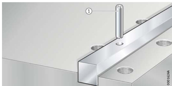
Figure 4 Fitting the square steel bar
