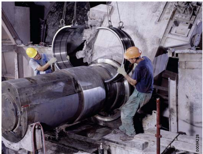
Figure 7 Mounting of a large split spherical roller bearing
