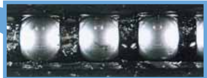
Detail view of the ball cage
