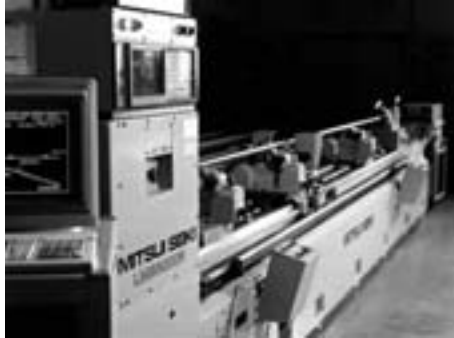
Automatic lead-measuring machine using laser
